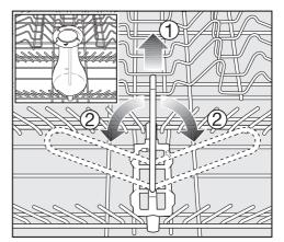
If the bottle holder is not needed, lift it up (1) and fold the sides down (2), as illustrated.
