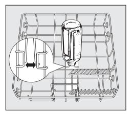
It can be inserted into the bottom basket in more than one place. See the areas marked in white in the illustration.
