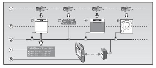
These instructions are for a communication enabled dishwasher that can be linked into the Miele@home system via a communication module (optional accessory).
